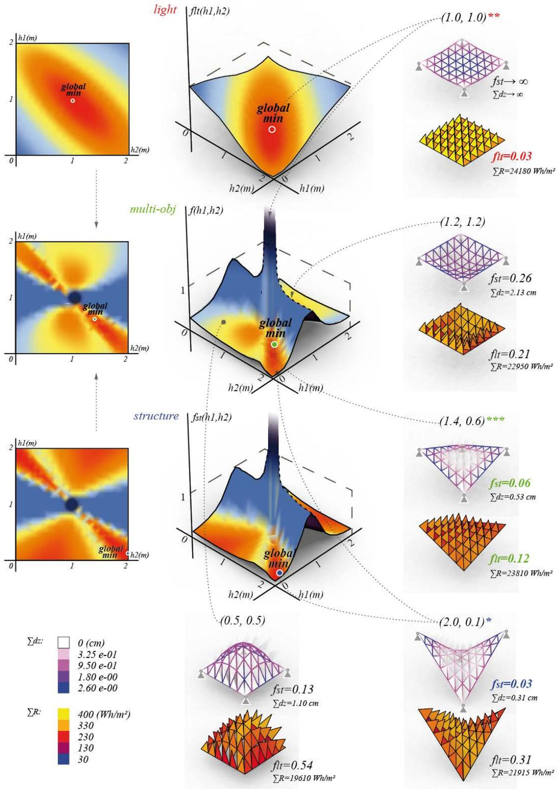
Figure 3. Left & centre: Landscape solution domains in 3-dimensions and in plan view. Right & bottom: Geometry population described for the structural ( $f_{st}$ ) and solar ( $f_{it}$ ) fitness. The spatial configurations are identified within each domain, if significant. Structural optimum\* has been reached for  $(h1, h2) = (2.0, 0.1)$ . Solar optimum\*\* for  $(h1, h2) = (1.0, 1.0)$ . Multi-objective optimum\*\*\* for  $(h1, h2) = (1.4, 0.6)$ .
