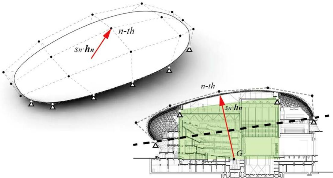
Figure 5. Esplanade parameterization. The control points  $n$ -th are governed by  $s_n \cdot \mathbf{h}_n$ . Top: parameterized geometry. Bottom: longitudinal section, the green geometry defines the control volume (free space). The black dashed line shows that the structure lies on a skewed plane.
