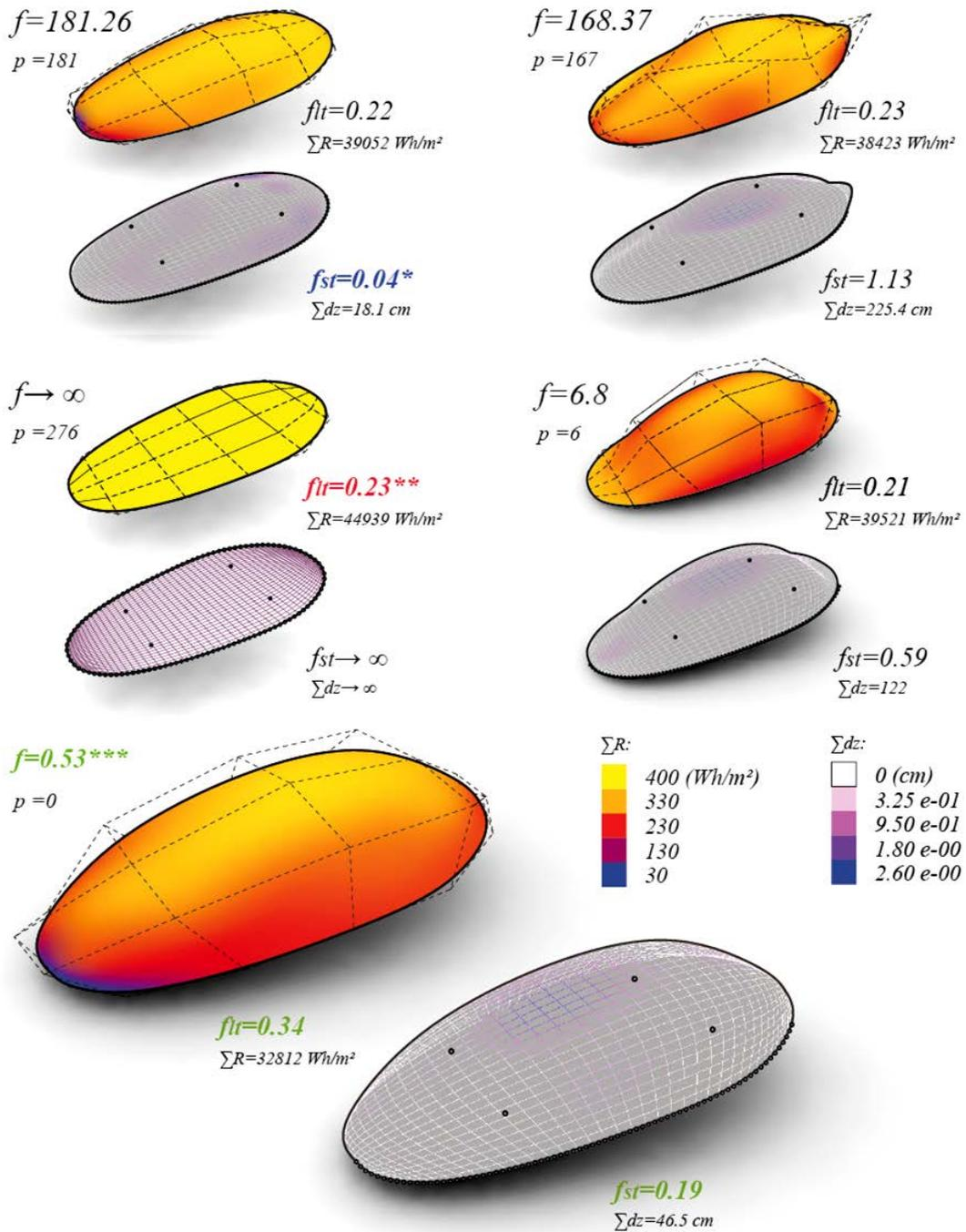
Figure 6. Some elements of the geometry population. Top left: the structural optimum\* interferes with the control volume. Middle left: solar optimum\*\*. Bottom: multi-objective optimum. Since 15 genes are processed, it is impossible to produce a graphic representation of the landscape solution domain.
