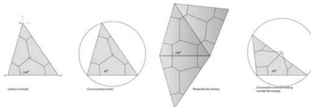
Fig. 3.2 The perpendicular meeting achieved by using circumcircle, and the problem when the corner angle exceeds 90 degree.
