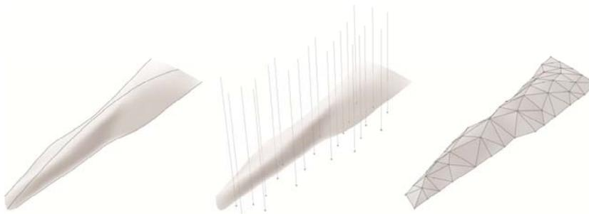
Fig. 3.1 From smooth surface to Delaunay mesh
