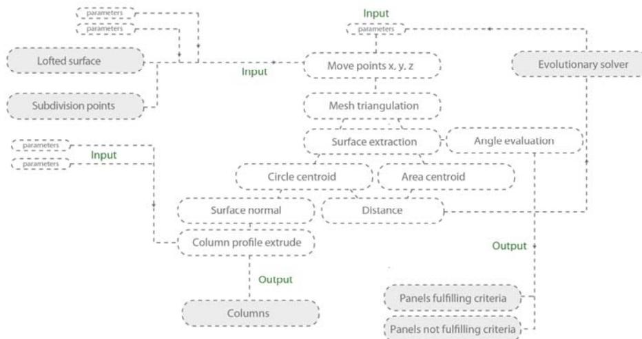
Fig. 4.1 Flow-chart of the optimization algorithm
