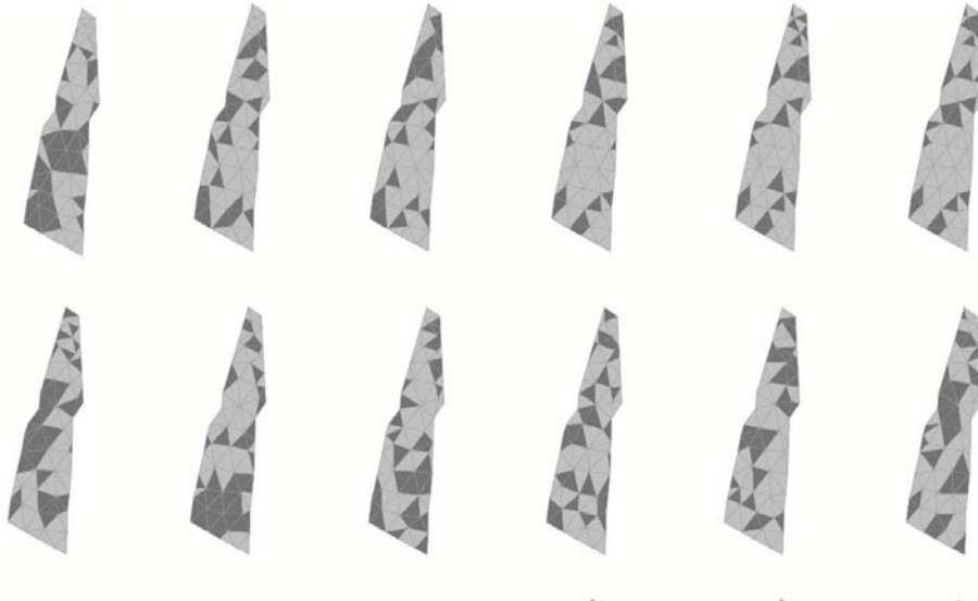
**Fig. 5.1** Process of optimization, dark facets is the non-successful triangles
